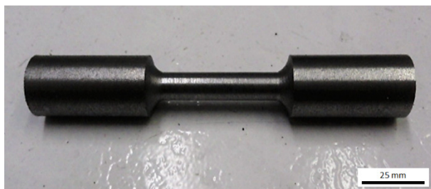
Figure 4. A test specimen for the mechanical test.
