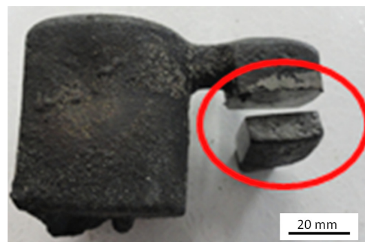
Figure 3. A test specimen for metallography.
