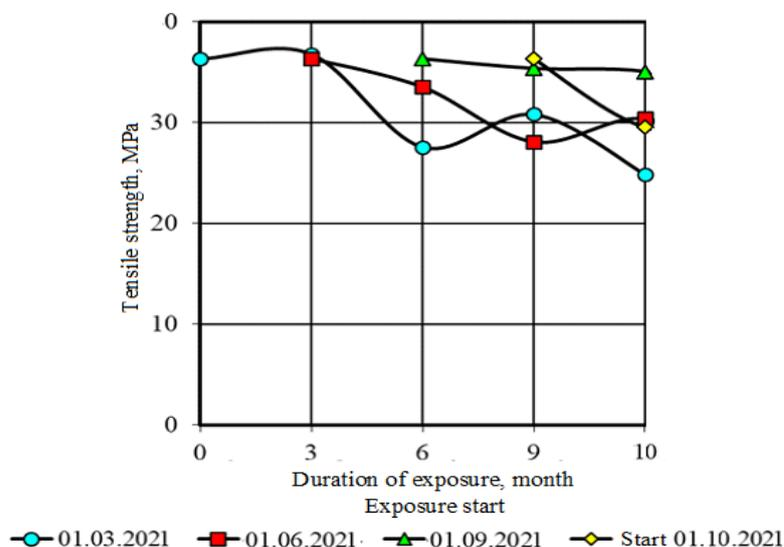
**Figure 2.** Change in tensile strength of specimens of composition Etal-247 + Etal-45M under tension relative to the common time axis
