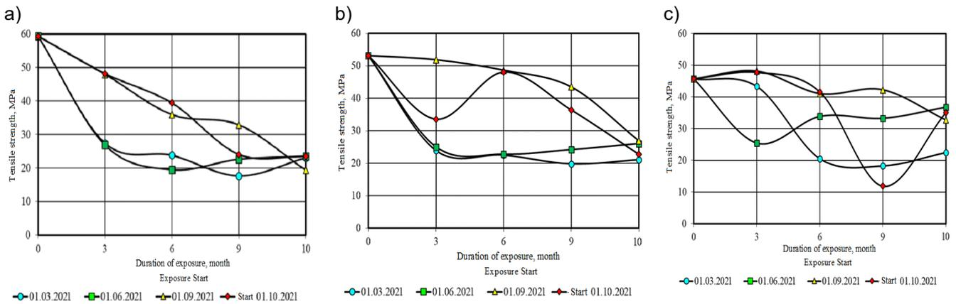
**Figure 3.** Change in the ultimate strength of specimens modified by Etal-1, depending on the season of the beginning of exposure (a - ED-20 + Etal-45M; b - (90% ED-20 + 10% Etal-1) + Etal-45M; c - (75% ED-20 + 25% Etal-1) + Etal-45M).
