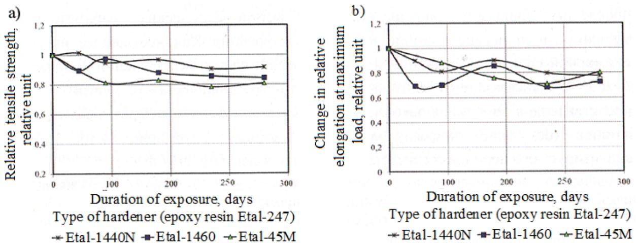
**Figure 8.** Change in the relative ultimate strength (a) and relative elongation (b) during stretching of an epoxy polymer based on modified Etal-247 resin, depending on the duration of natural exposure
