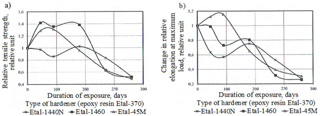
**Figure 6.** Change in the relative ultimate strength (a) and relative elongation (b) during stretching of the epoxy polymer based on the modified Etal-370 resin, depending on the duration of full-scale exposure
