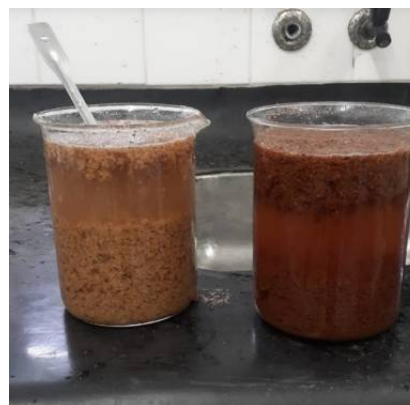
Figure 7. Whashing the samples with reagent water type IV.
