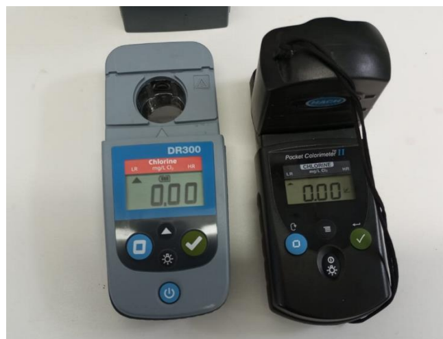
Figure 2. DR300 Pocket Colorimeter (left) and POCKET Colorimeter II Colorimeter for Chlorine analysis.
