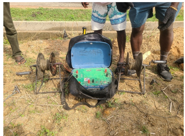
Figure 3. A resistivity meter was employed for the survey
