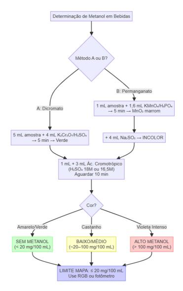
**Figure 2.** Flowchart of Brazilian colorimetric methods for methanol determination in alcoholic beverages. The method offers two oxidizing routes (A: dichromate or B: permanganate), both followed by a chromogenic reaction with chromotropic acid. The violet color intensity is proportional to methanol concentration, allowing visual screening or quantification with portable devices.
