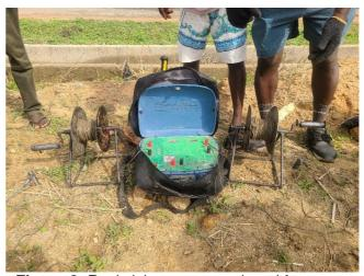
Figure 3. Resistivity meter employed for survey
