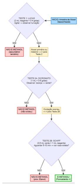
**Figure 1.** Flowchart of the combined analysis protocol for methanol detection in alcoholic beverages using classical methods. The process consists of initial screening with Lucas Test (elimination of secondary and tertiary alcohols), followed by dichromate oxidation and specific confirmation with Schiff's reagent.
