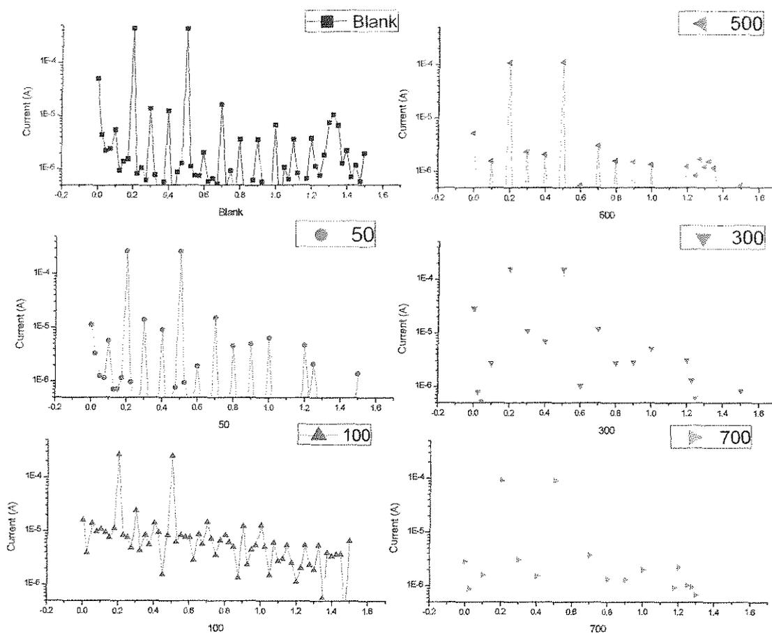
Figure 8. Intermodulation spectrum for Carbon steel in 1 M HCl solutions without and with various concentrations (50-700 PPM) of Zygophyllum Album at 25°C.
