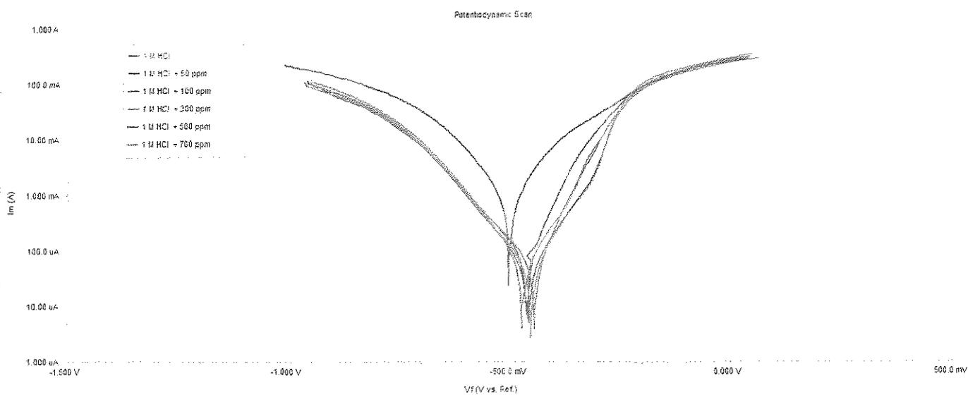
Figure 4. Potentiodynamic polarization curves for Carbon Steel in 1M HCl solution without and with various concentrations (50-700 PPM) of Zygophyllum Aegyptium at 20°C.
