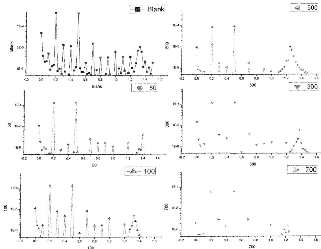
Figure 9. Intermodulation spectrum for Carbon steel in 1 M HCl solutions without and with various concentrations (50-700 PPM) of Zygophyllum aegyptium at 25°C.
