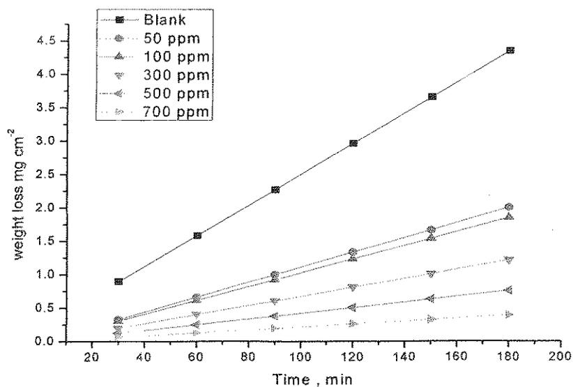
Fig. 2. Weight loss-time curves for the dissolution of N80 Carbon steel in the absence and presence of different concentrations of *Zygophyllum aegyptium* at 25 °C
