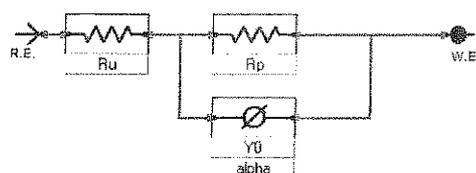
Figure 7. Electrical equivalent circuit used to fit the impedance data.
