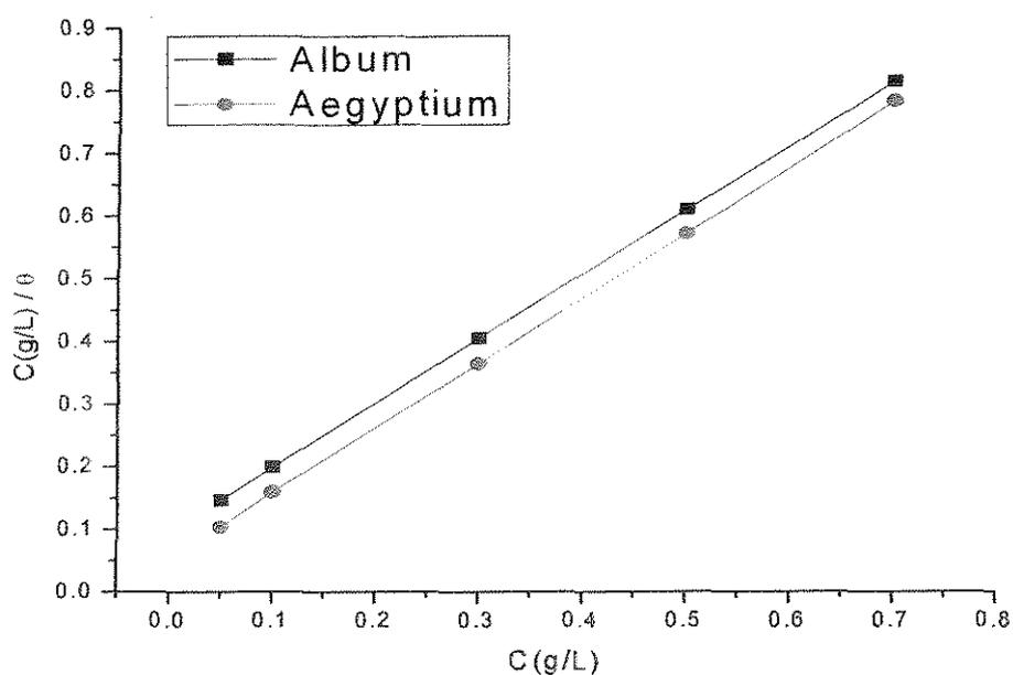
Figure 10 . Curve fitting of corrosion data for N80 carbon steel in 1M HCl in the presence of different concentrations of Zygophyllum album and Zygophyllum aegyptium extracts to Langmuir adsorption isotherm at 25° C.
