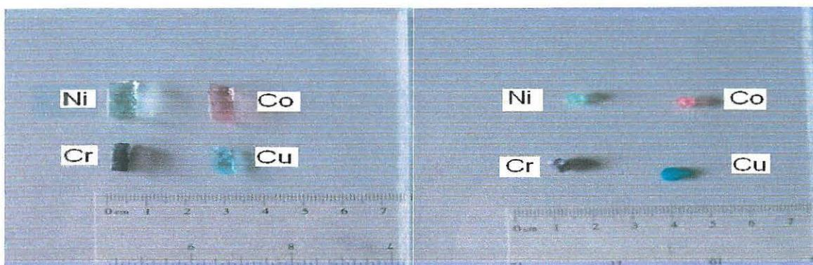
Figure 3. Pre-shrunk polymer gels with metallic nitrates (L) and shrunken gels (R)
